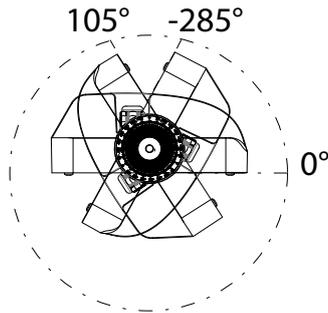
Unacceptable luminaire mounting - light is not supposed to be directed at luminaire and its parts.
