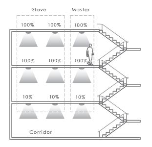
3. The person walks to the 3rd floor; the 3rd master switches the light on 100%. All slaves on the 3rd floor turn the light on and the master on the 4th floor switches on at standby level. Meanwhile, the lights on the 1st floor are dimmed to stand-by level after hold-time
