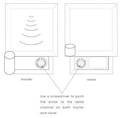
Channel "0" is not for fast grouping, and sensors can only be grouped by remote control with this channel.
