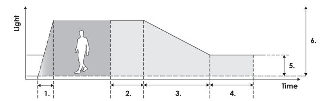
For optimum adjustment to a variety of situations, there is a choice of different profiles that are defined by a few parameters:
