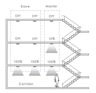
1. While the 1st sensor detects motion on the 1st floor, it switches the light on at 100% and sends signal to all slave units. All slaves on the 1st floor turn on and the master on the 2nd floor switches on at stand-by level.
