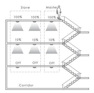
4. The person walks to the 4th floor; the 4th master switches the light on at 100%. All slaves on the 4th floor turn the light on. Meanwhile, all sensors on the 1st floor turn the light off after stand-by period, and all lights on the 2nd floor dim to stand-by level after hold-time.
