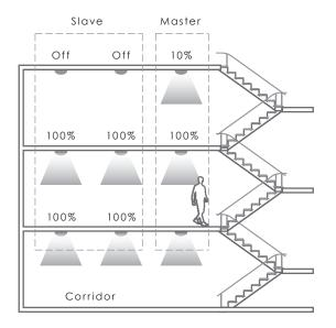
2. The person walks to the 2nd floor; the 2nd master switches the light on at 100%. All slaves on the 2nd floor turn the light on and the master on the 3rd floor switches on at stand-by level.
