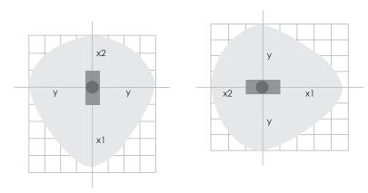
For motion detection PIR technology is used. PIR Lens is made to detect moving people in working areas with the following performance criteria:
