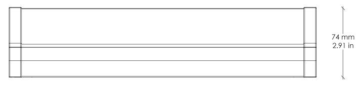
$320/600/880/1160 \ \text{mm} \ | \ 12.60/23.62/34.65/45.67 \ \text{in} \ - \text{dimensions without sensor} \ 405/685/965/1245 \ \text{mm} \ | \ 15.94/26.97/37.99/49.02 \ \text{in} \ - \text{dimensions with sensor} \$
