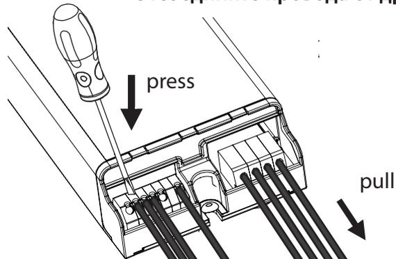
**5** Unscrew the LED driver, replace it and put it back into place
