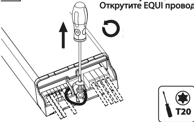
**4** Disconnect the wires from the driver
